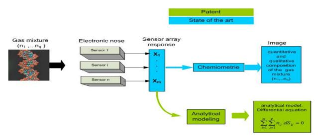
The derived models are equations in differential form ,which connect the number of moles nj of the mixture component j to the partial sensitivities sij of the ith sensor array element, when it interacts with the j constituents of the gaseous mixture.
